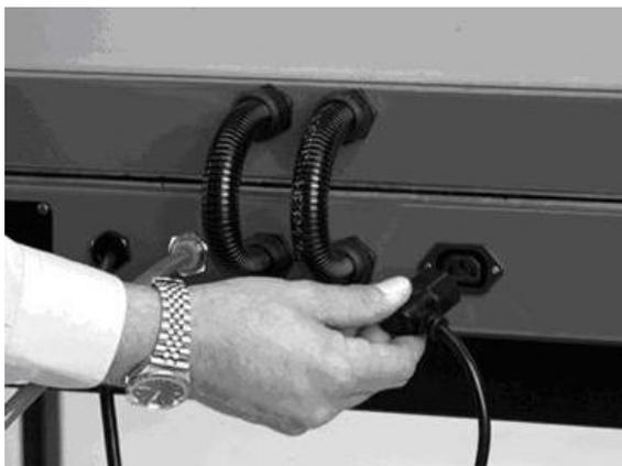
The electrical lead from the pump can now be connected to the socket in the rear of the press.
