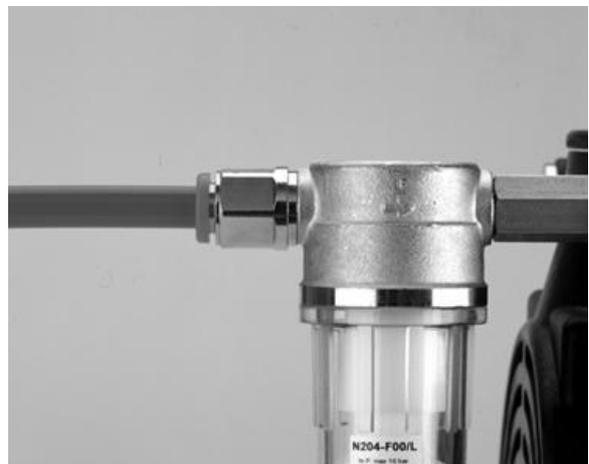
Should you need to remove a tube from a connector, simply push down on the rim of the fitting with a finger and the tube should easily pull out.
