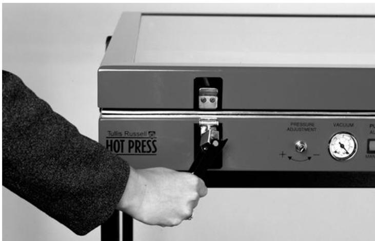
The catch is designed to work with a light “click”. Adjusting it to make it excessively tight will not improve the effectiveness of the vacuum seal, and may seriously damage the catch.
