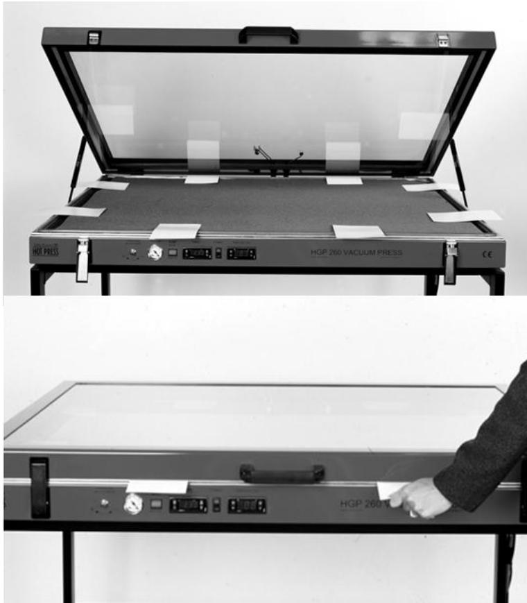
6. Search for a hole in the diaphragm. Splits are most common along the edges and corners. Switch off power supply to press. Remove the screws holding the diaphragm. Then lift it out of the press and inspect both sides for holes.
